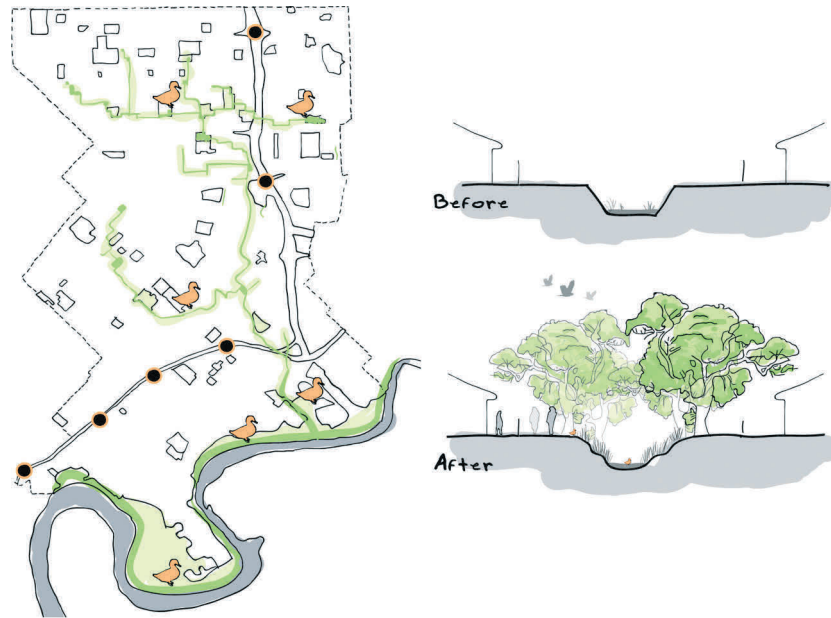
Figure 11. The Green Stream: In this concept, tree planting was focussed in streets around upgraded drains and foreshores in a bid to retrofit Water Sensitive Urban Design to Bayswater's extensive matrix of drains which currently only serve flood mitigation functions.
